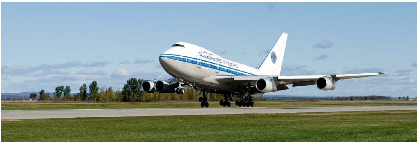
Pratt & Whitney 747SP flying test bed (FTB) in PurePower Engines livery. It will test PW1000G engines for the Bombardier CSeries, Airbus A320neo, and Irkut MC-21 aircraft families.
