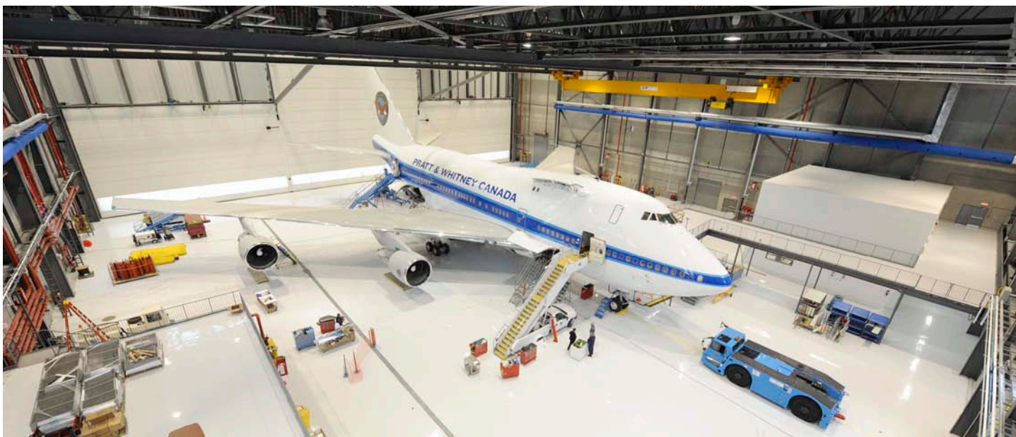
The new Pratt & Whitney Canada 747SP flying test bed (FTB). It will test the PW1000G engine for the Mitsubishi Regional Jet (MRJ), as well as the PurePower PW800 engine series, for the next generation of large business jets.
